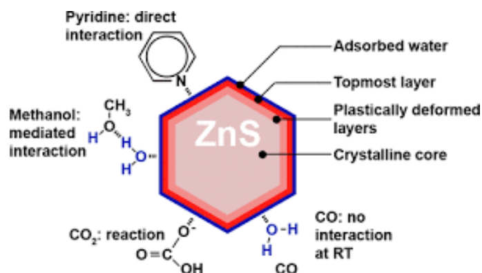
FIGURE 2 Core-shell structure and surface interaction of ZnS nanoparticles
